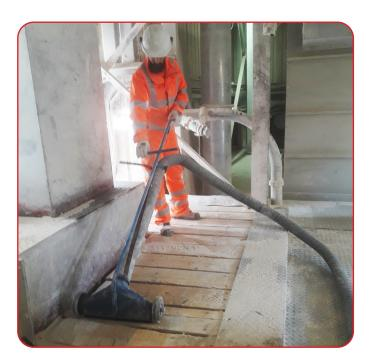
A wide range of accessories allows the operators to quickly and easily remove spillages even in the most hard to reach areas.
